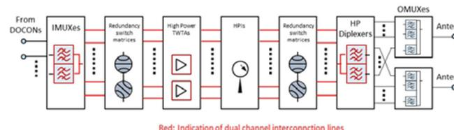
Fig. 3: Block diagram for dual channel operation
