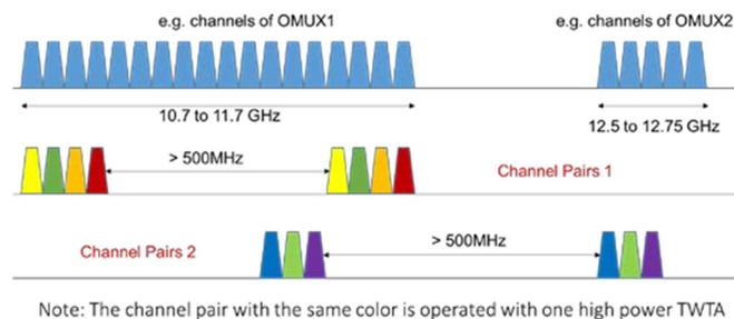
Fig. 2: Channel frequency scheme for dual channel concept
