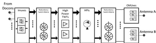
Fig. 1: Traditional architecture of DTH applications.
