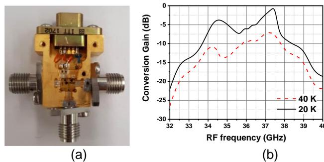
Fig. 2. (a) photo of the packaged mixer module, and (b) its measured conversion gain.
