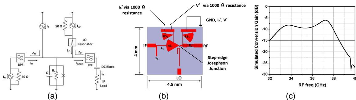
Fig. 1. (a) schematic model of the HTS MMIC Josephson mixer; (b) the circuit layout, and (c) its simulated frequency response of conversion gain.
