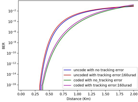
Fig. 1. BER with 4bps/Hz at 100GHz
