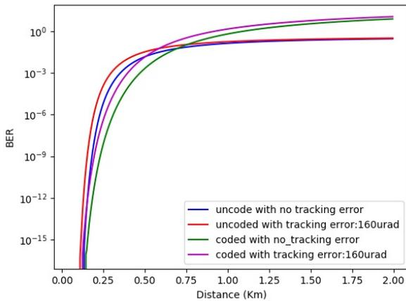
Fig. 2. BER with 4bps/Hz at 200GHz
