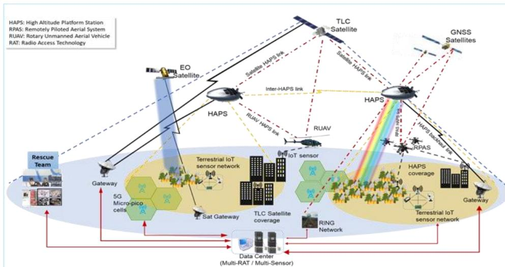
Fig. 1 Advanced Solution Architecture for integrated Earth & Space disaster management services
