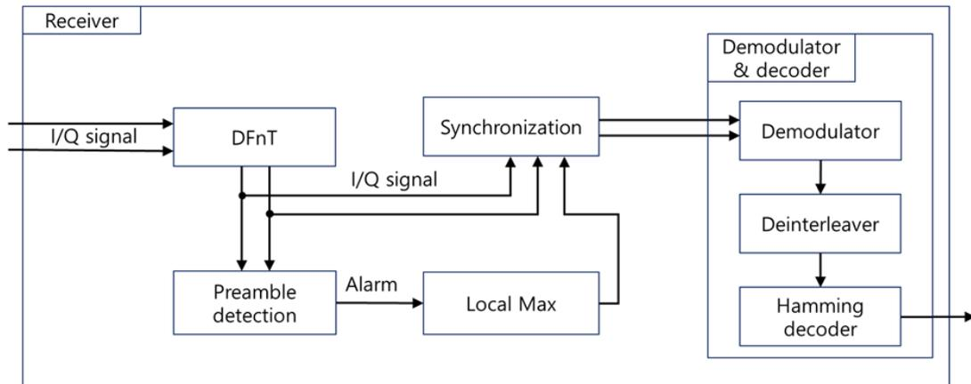
**Figure 2. Receiver block diagram**
